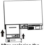
After replacing the batteries, put the battery box back to original location and screw it tightly.
