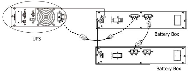
**NOTE:** Maximum connected external battery boxes up to 4 units.
